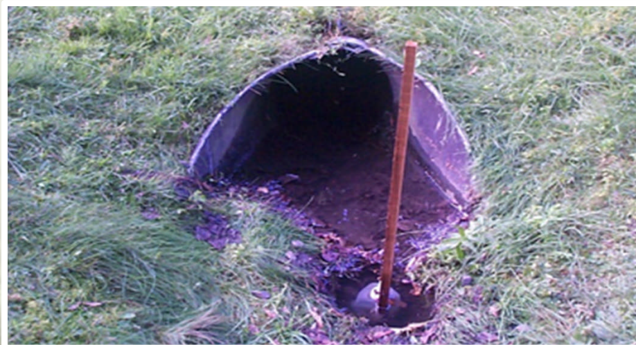
Sampling outfall using Passive Sampler .
